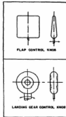
(b) Powerplant control knobs must conform to the general shapes (but not necessarily the exact sizes or specific proportions) in the following figure:
