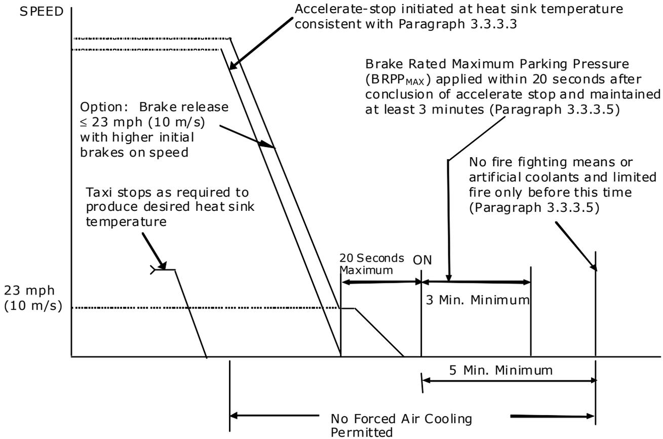
**Figure 3-1. Taxi, Accelerate-Stop, Park Test Sequence**
