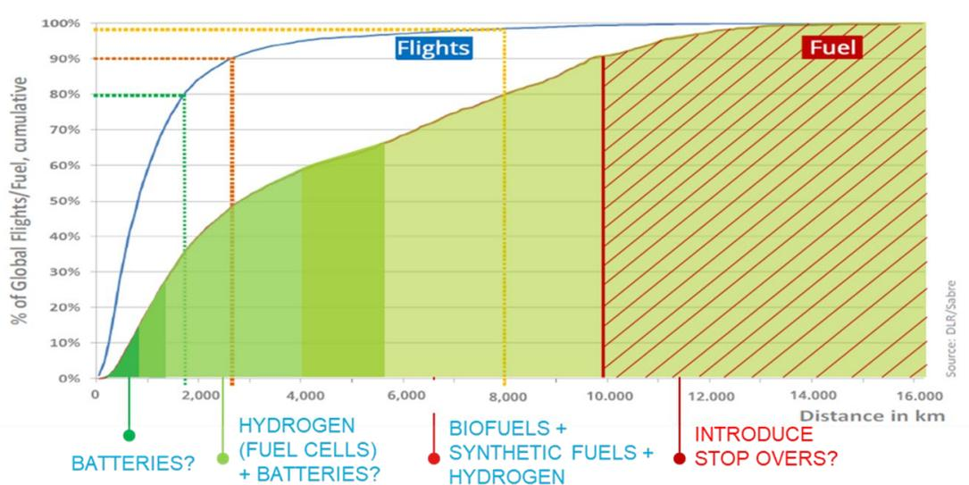
From this graph, it can be concluded that electrified flight is not (yet) a serious option for large distances, simply because batteries contain less energy/kg than Jet A1. Electric powered aircraft are thus limited on their range
