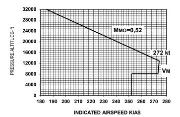
AIRSPEED LIMITS (IAS) Maneuvering  $(V_A)$  - sea level: 370 km/h (200 kias) (Cont.) Flaps extended  $(V_{FE})$
