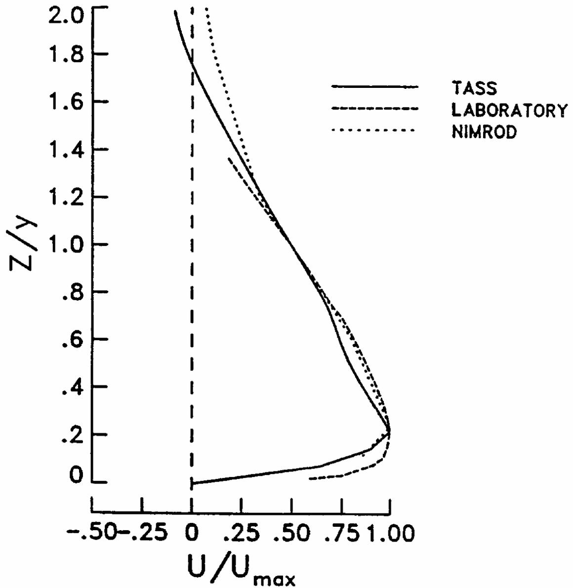
Figure 2 Vertical Profile of Microburst Outflow (Nondimensional)
