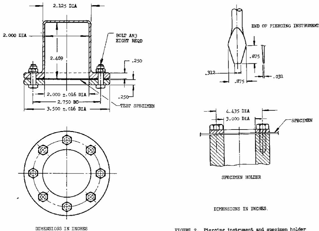
FIGURE 1. Permeability cup assembly
