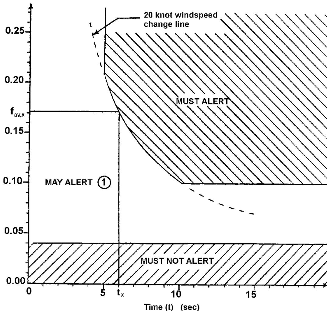
$f_{av,x}$  = average shear intensity to cause a warning at time  $t_x$  (resulting in a 20 knot windspeed change, bounded as shown; applies to horizontal, vertical, and combination shear intensities)
