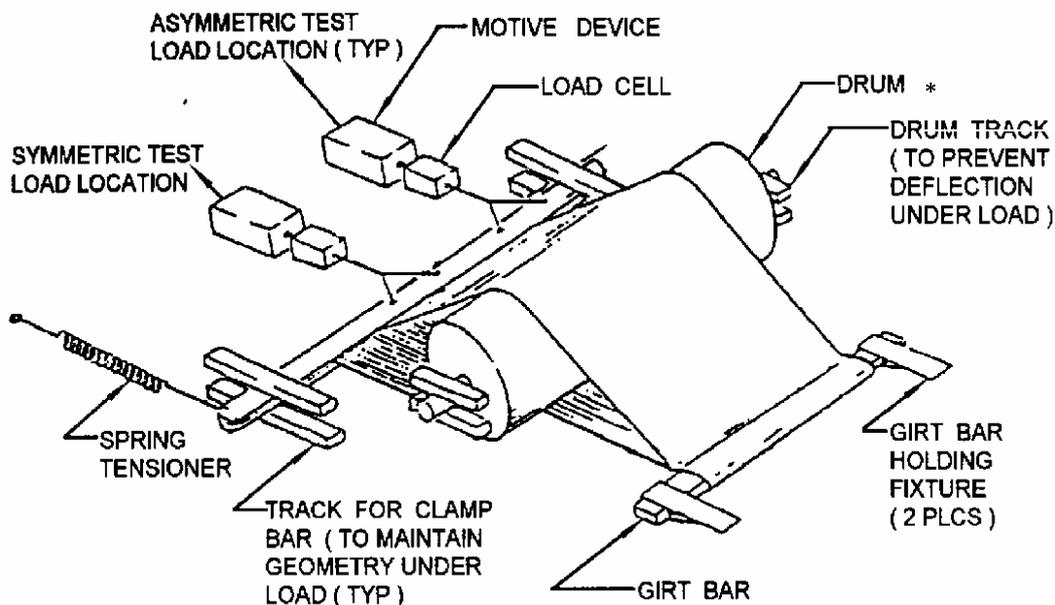
\* DRUM SHALL RETAIN ITS SHAPE THROUGHOUT TEST LOADING AND SHALL BE OF SUFFICIENT DIAMETER TO ALLOW SIMULATION OF THE GIRT ATTACHMENT ANGLE, A.
