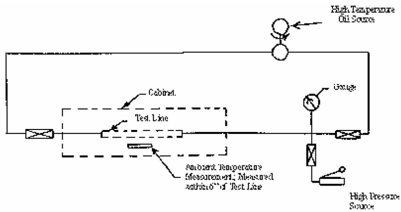
Typical Setup for High Temperature Pressure Testing
