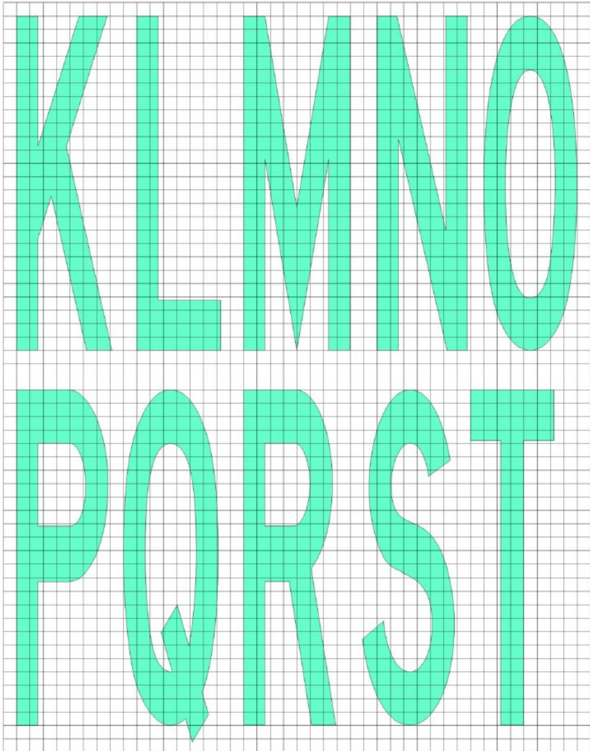
Figure L-10B. Mandatory instruction marking inscription form and proportions
