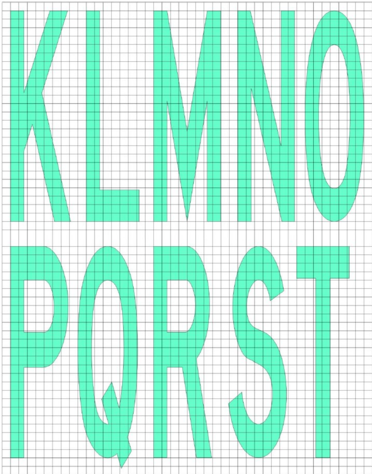
Figure L-10B. Mandatory instruction marking inscription form and proportions
