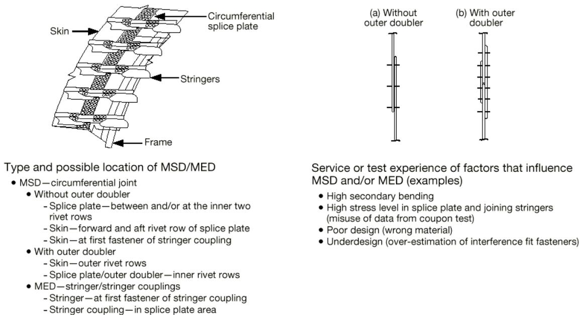
**Figure A2-2: Circumferential joints and stringers (MSD/MED)**
