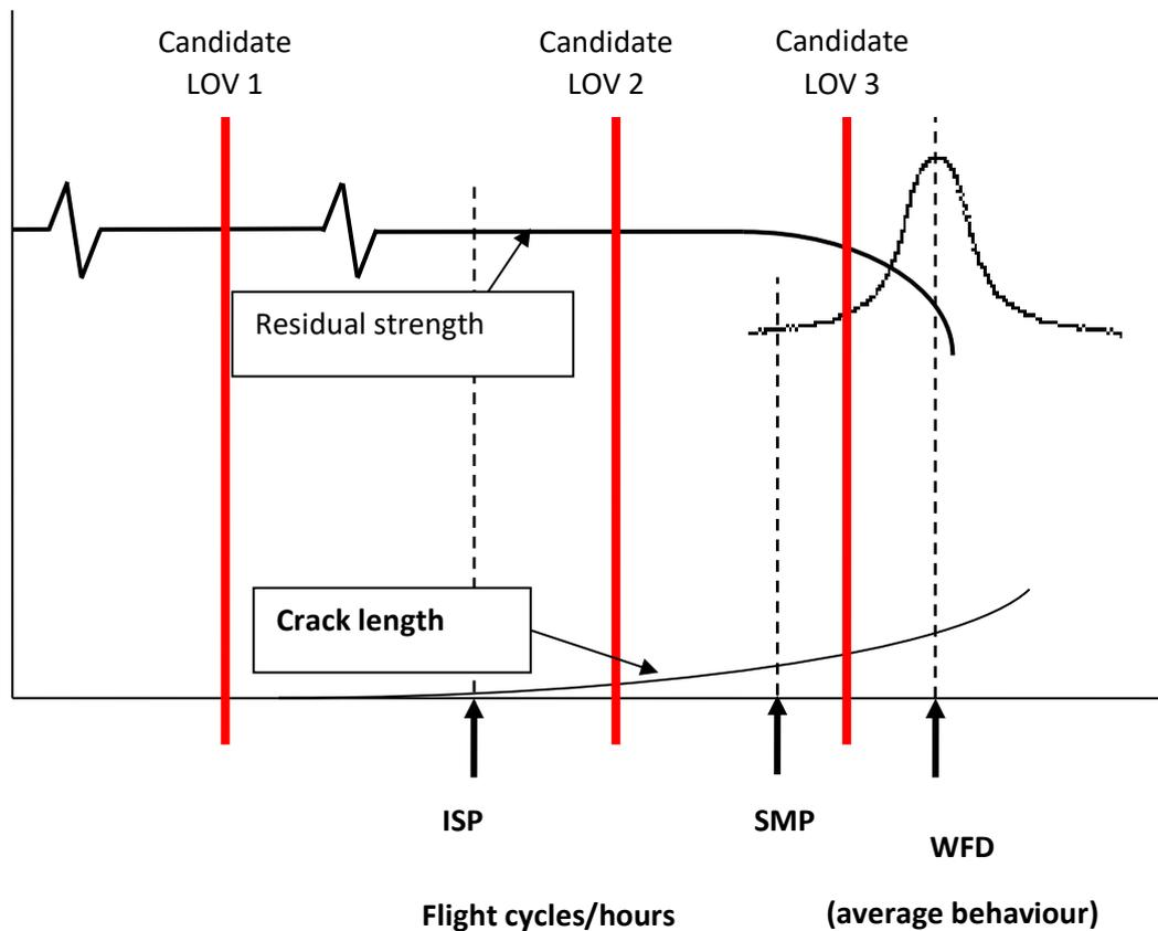
**Figure 2-1: Comparison of WFD-susceptible structure to aircraft LOV**
