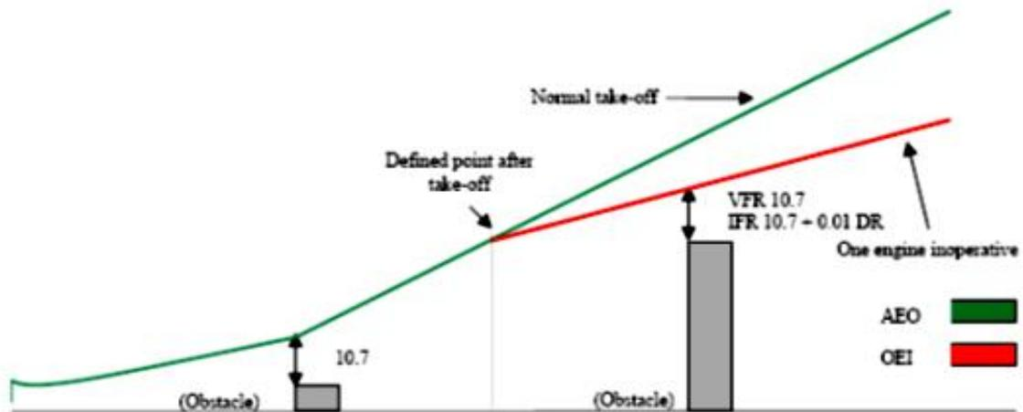
Figure 4: Performance Class 2 Obstacle Clearance (plan view)
