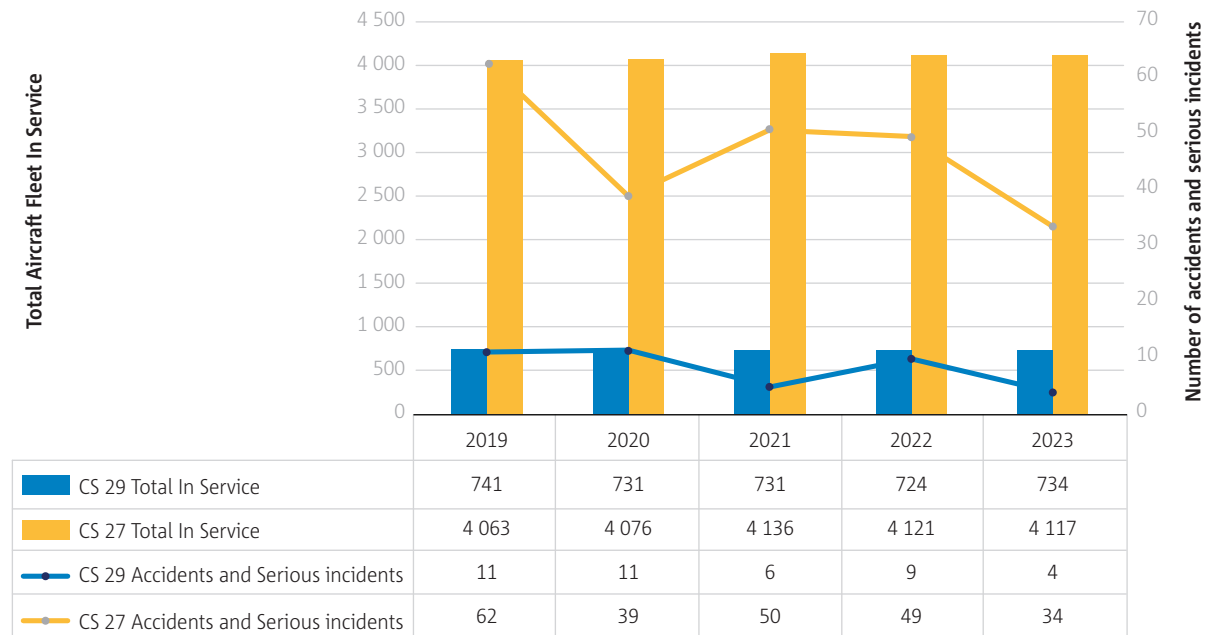
► Figure 3.7 Accidents and serious incidents by certification specification for all helicopter operations with the breakdown of aircraft certification type for the reported fleet
