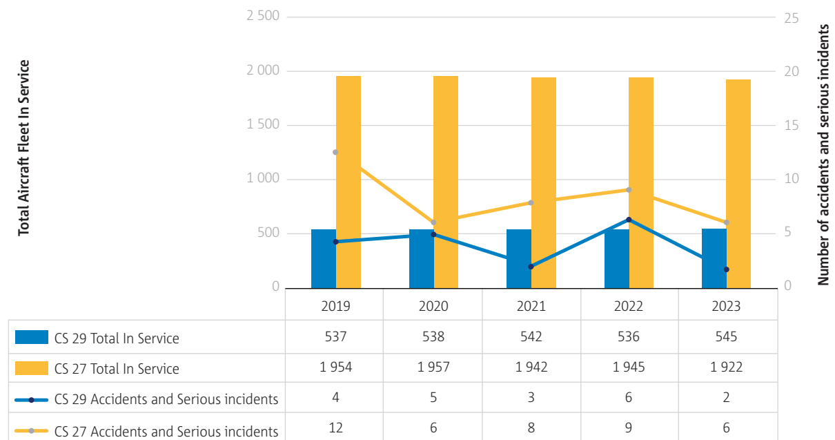
► Figure 3.17 Accidents and serious incidents by certification specification (CS27/CS29) for CAT operations with the breakdown of aircraft certification type for the reported fleet
