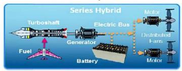
A system where only the electric motors are connected to the fans, and the gas turbine engine is used to drive an electrical generator which drives the motors and/or charges the batteries
