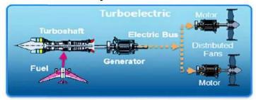
A system that relies fully on gas turbines to drive electric generators which then power inverters and motors to drive disturbed fans
