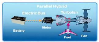
A system that uses a battery-powered motor and gas turbine engine both mounted on a shaft that drives fan, so one or both can provide propulsion at any given time
