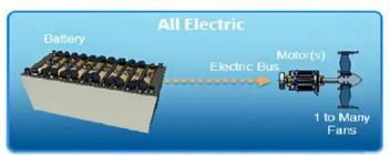
All-electric aircraft systems use batteries as the only source of propulsion power
