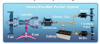
A system with one or more fans that can be driven directly by a gas turbine engine, and additional fans that are driven exclusively by electrical motors which can be powered by a battery or a turbine-driven generator
