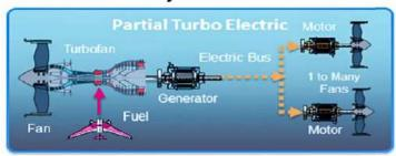
A system that uses electric propulsion to provide part of the propulsive power, with the rest provided by a turbofan driven by a gas turbine
