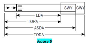
(6) When intersection take-offs are performed, the datum line from which the reduced runway declared distances for take-off are determined, shall be defined by the intersection of the downwind edge as shown in the figure below:
