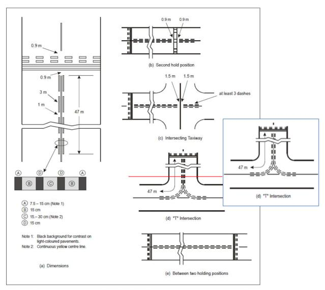
Figure L-6. Enhanced taxiway centre line marking
