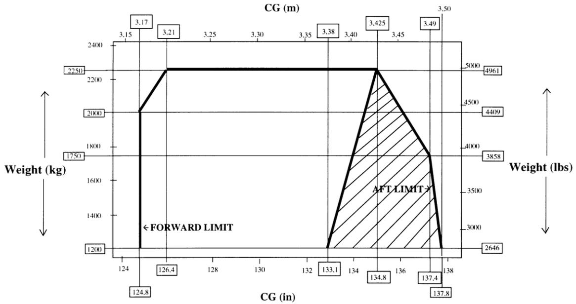
13.4 Longitudinal C.G. limits for AS 350 B3 Arriel 2D a/c incorporating modification OP-3369:
