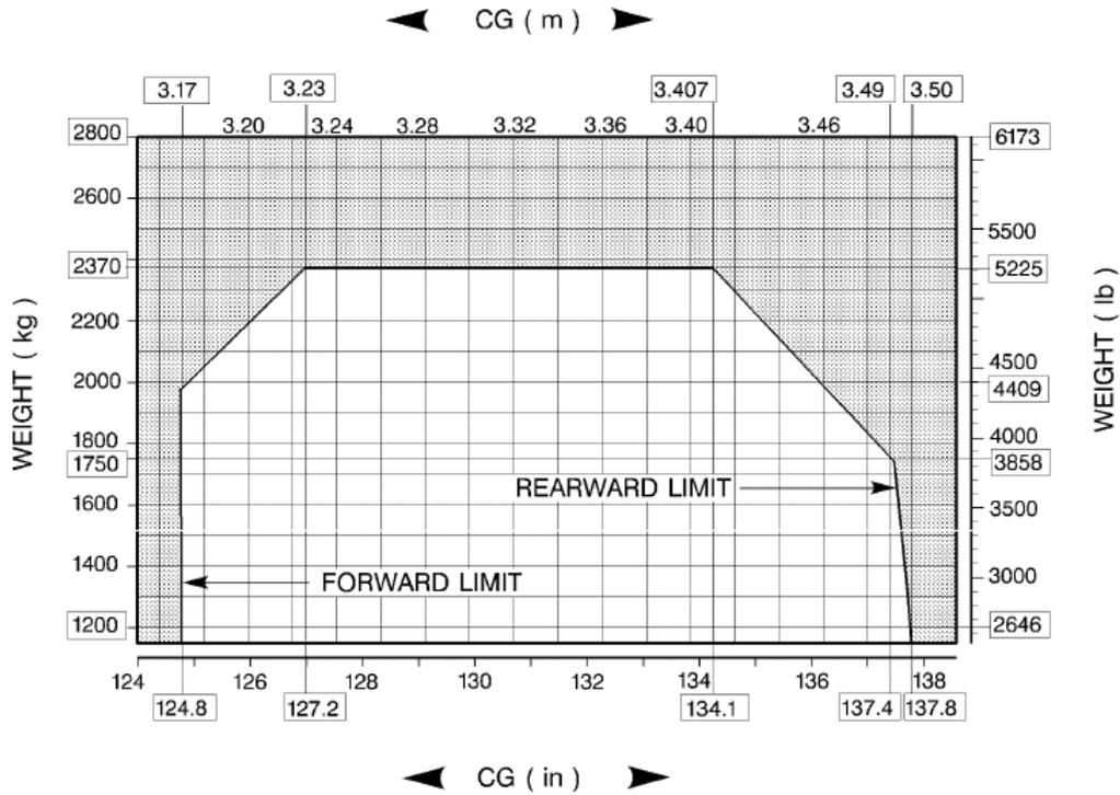
13.2 Longitudinal C.G. limits for AS 350 B3 Arriel 2B (before modifications AMS 072803 and 072808), and for AS 350 B3 Arriel 2B1
