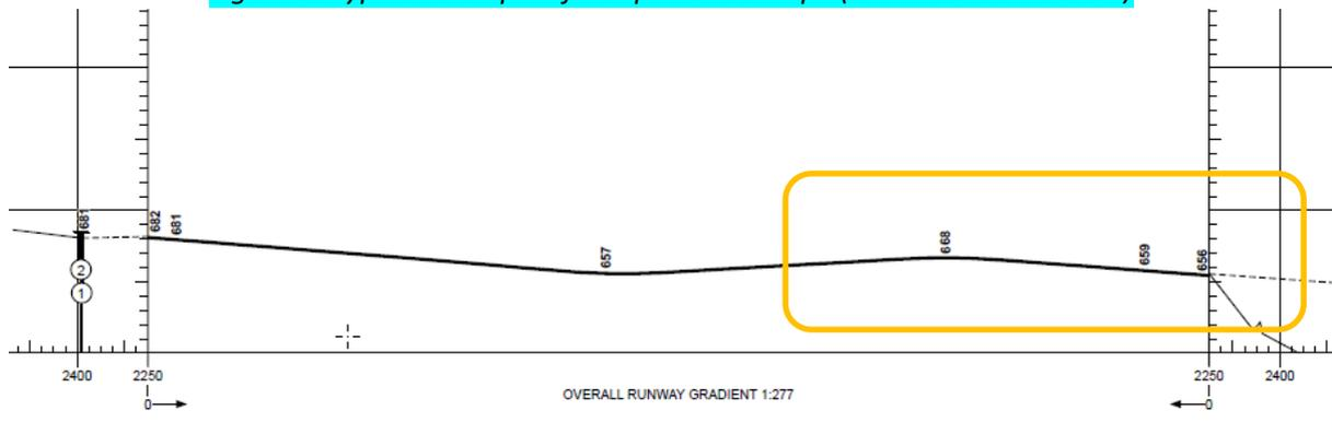
Figure 3: Typical example of 'moderate' LSAA slope due to variation around mean LSAA slope greater than 1 m but lower than 2 m (EGNM 32 dated 2018)
