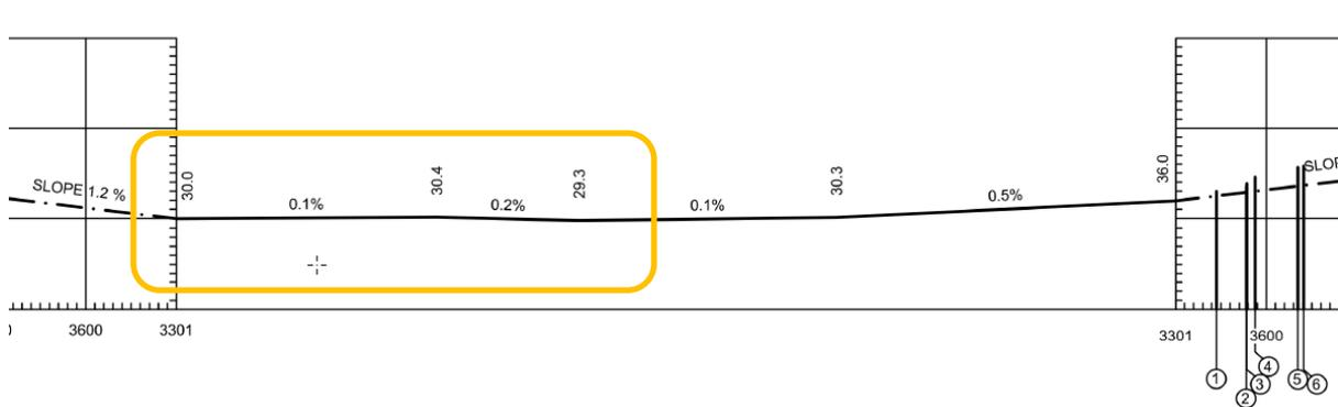
Figure 2: Typical example of 'simple' LSAA Slope (ESSA 01L dated 2018)
