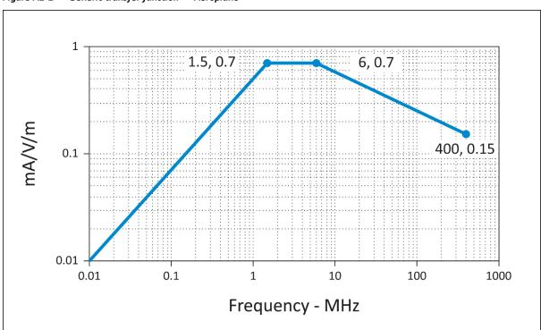
Generic transfer function normalised to 1 V/m for an aeroplane with a fuselage length of > 25 m and  $\leq$  50 m.
