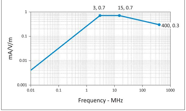
Generic transfer function normalised to 1 V/m for an aeroplane with a fuselage length of  $\leq 25 \text{ m}$ .
