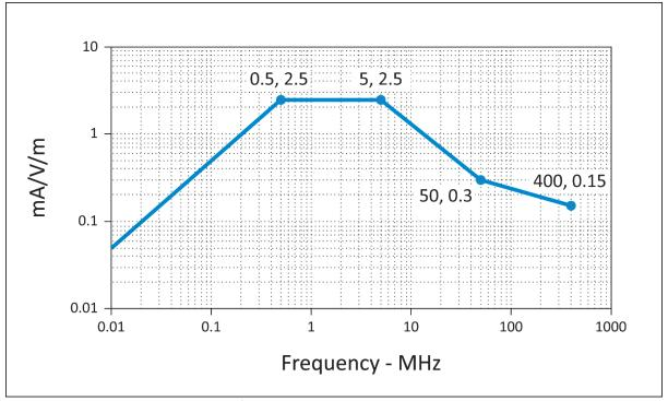
Generic transfer function normalised to 1 V/m for an aeroplane with a fuselage length of > 50 m.
