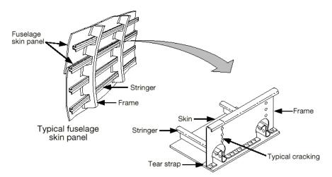
• MED-the cracking of frames at stringer cutouts at successive longitudinal locations in the fuselage. The primary concern is for those areas where noncircular frames exist in the fuselage structure. Fractures in those areas would result in panel instability.
