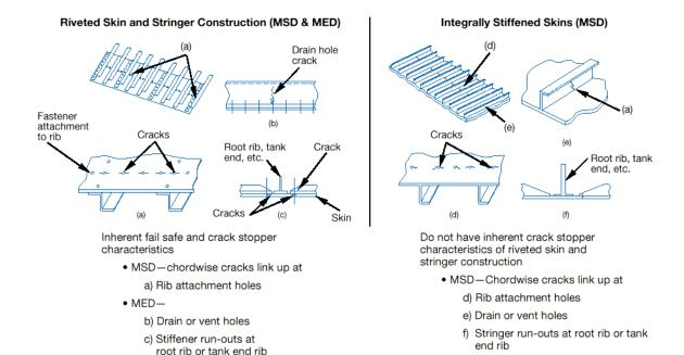
Figure A2-16 Typical Wing and Empennage Construction (MSD/MED)
