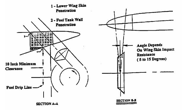
FIGURE 2 - DRY BAY SIZING DETERMINATION EXAMPLE
