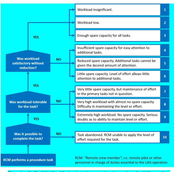
Figure 1 — Bedford Workload Scale adapted to operational procedures for UAS operations
