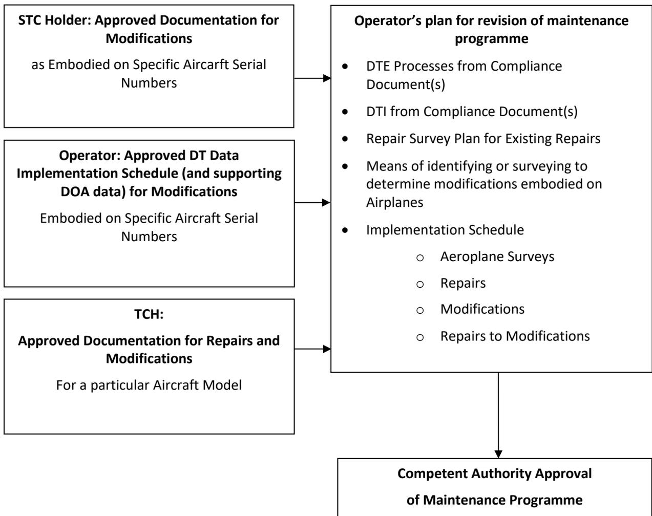
Figure A3-2 - Operator's Maintenance Programme Approval Process
