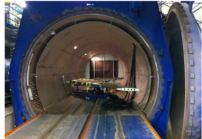
Thermal test on the instrumented horizontal stabilizer static and FDT component test article
