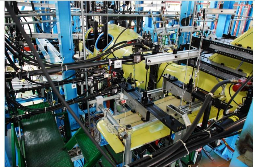
FIGURE 12.8.5.4(e). KC-100 full-scale fatigue setup
