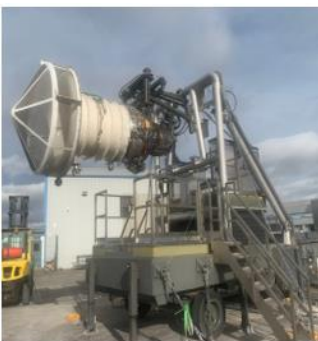
Picture of the LF507/ALF502 test stand (left) and PW127G (Airbus C-295) test probe
