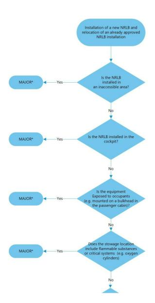
\* Any subsessequent relocation of equipment containing a battery with ETSO C142b authorisation may be classified as minor provided that the change has no impact on the original Safety Assessment and the new conditions of installation are not worse than the original ones, in terms of separation to oxygen lines/equipment, water, fuel, other flammable substances, heat points, separation from occupants (in case of exposed installation)
