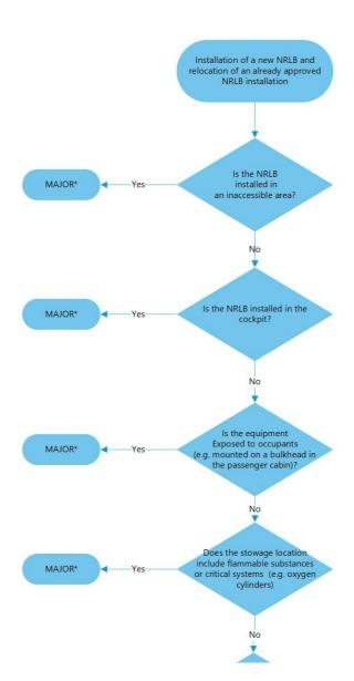
\* Any subsesequent relocation of equipment containing a battery with ETSO C142b authorisation may be classified as minor provided that the change has no impact on the original Safety Assessment and the new conditions of installation are not worse than the original ones, in terms of separation to oxygen lines/equipment, water, fuel, other flammable substances, heat points, separation from occupants (in
