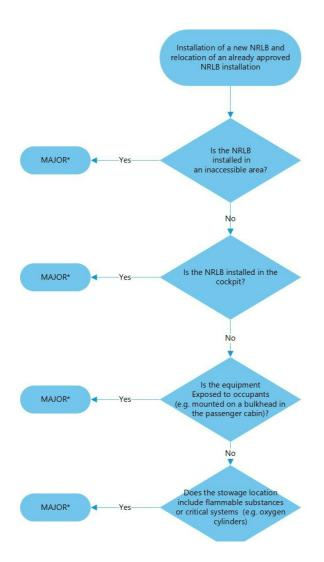
\* Any subsessequent relocation of equipment containing a battery with ETSO C142b authorisation may be classified as minor provided that the change has no impact on the original Safety Assessment and the new conditions of installation are not worse than the original ones, in terms
