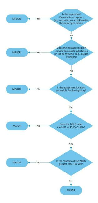
\* Any subsesequent relocation of equipment containing a battery with ETSO C142b authorisation may be classified as minor provided that the change has no impact on the original Safety Assessment and the new conditions of installation are not worse than the original ones, in terms of separation to oxygen lines/equipment, water, fuel, other flammable substances, heat points, separation from occupants (in case of exposed installation).
