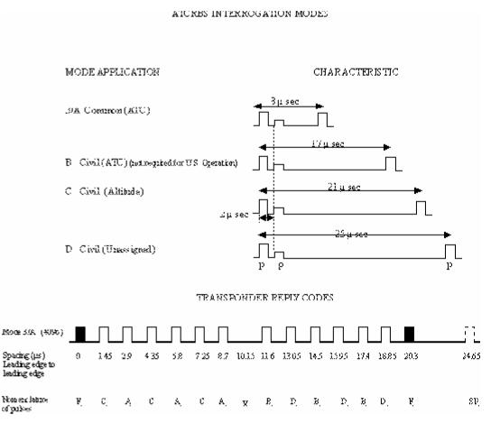
Figure 1 – ATCRBS, Interrogation modes and reply codes
