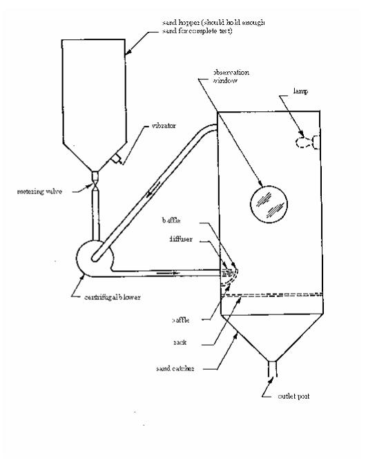
Figure 1. Schematic Sand Test Arrangement (Ref. Section 7.8)
