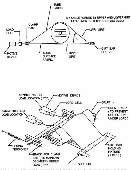
\* DRUM SHALL RETAIN ITS SHAPE THROUGHOUT TEST LOADING AND SHALL BE OF SUFFICIENT DIAMETER TO ALLOW SIMULATION OF THE GIRT ATTACHMENT ANGLE, A.
