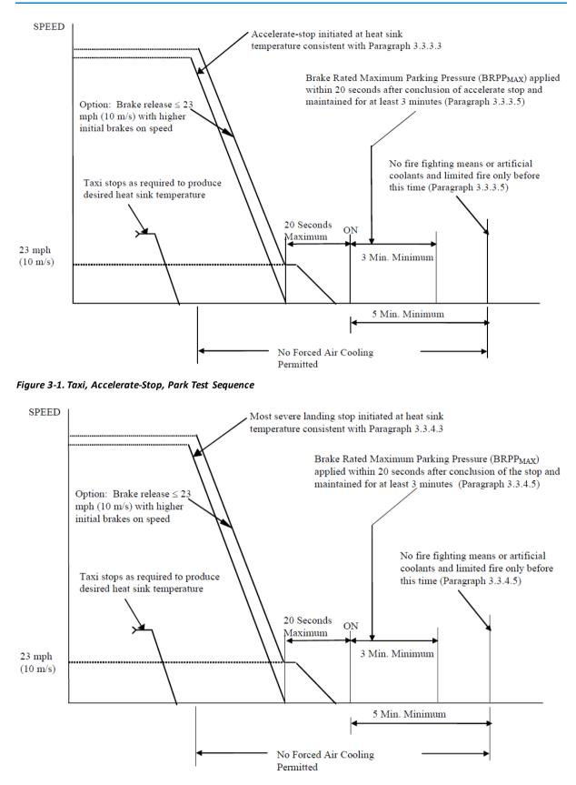
Figure 3-2. Most Severe Landing-Stop, Park Test Sequence
