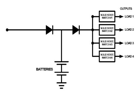
Figure A-2: An example BEPU Current Flow
