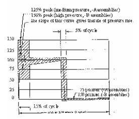
The curve shown above is the approximate pressure-time cycle determined to be of proper severity for impulse testing of hose assemblies. The pressure-time curve shall be confined to the shaded area indicated.
