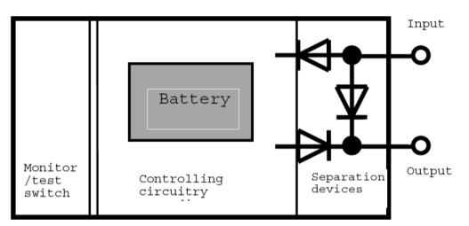
Figure A-1: BEPU Block Diagram
