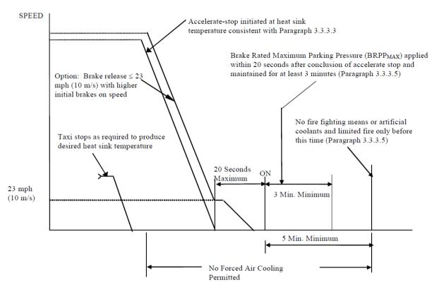
Figure 3-1. Taxi, Accelerate-Stop, Park Test Sequence
