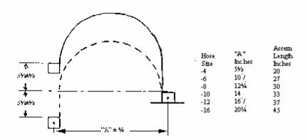
Assembly Flex Test Setup Figure III
