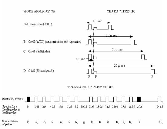
Figure 1 – ATCRBS, Interrogation modes and reply codes
