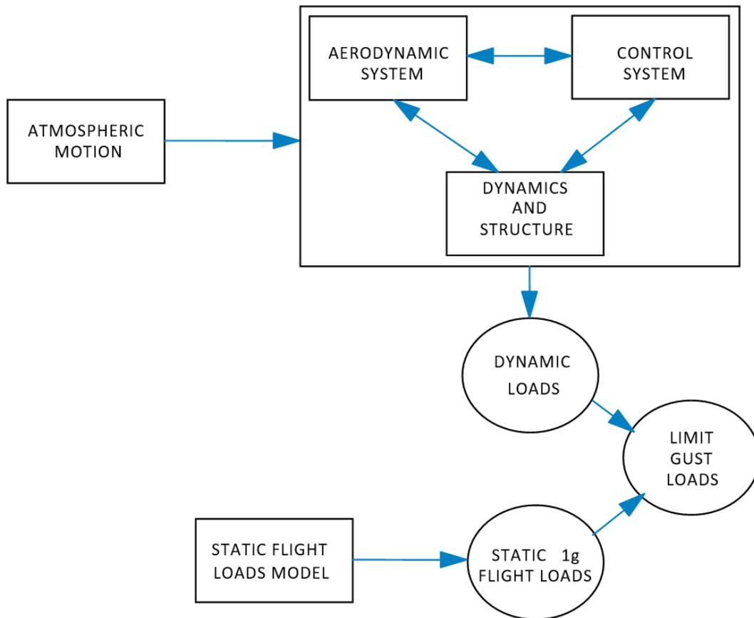
**Figure 1 Basic Elements of the Gust Response Analysis**
