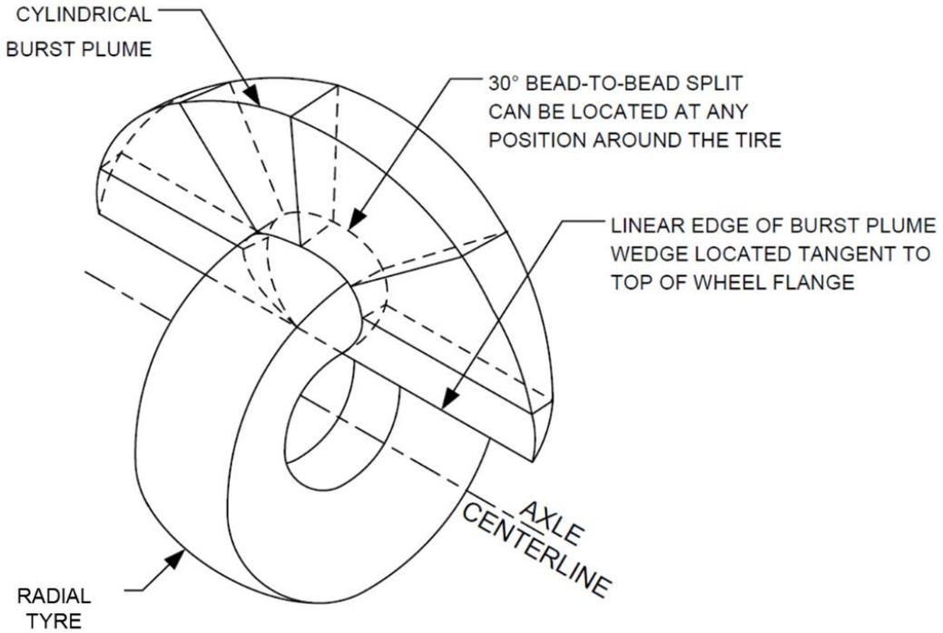
**Figure 4e – Tyre Burst Pressure Effect – Radial Tyre**
