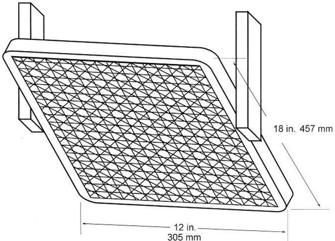
Figure 3b – Air Propane Radiant Panel
