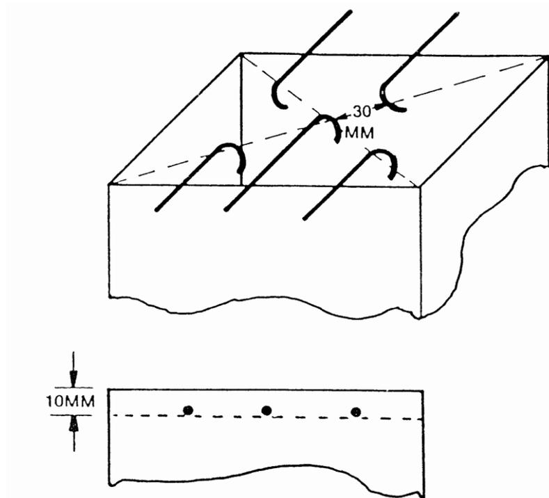
**FIGURE 5. THERMOCOUPLE POSITION**
