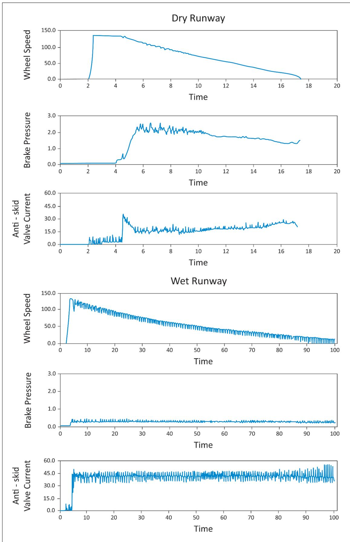
**FIGURE 3. ANTI-SKID SYSTEM RESPONSE CHARACTERISTICS Fully Modulating System**
