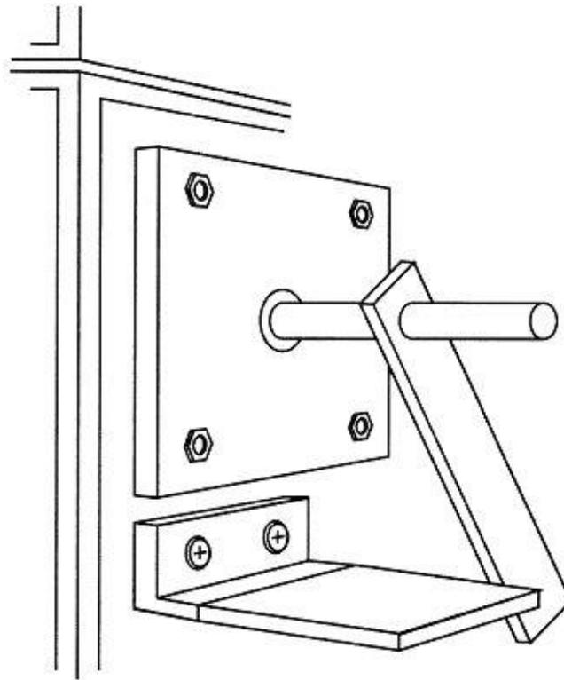
Figure 8 - Propane Burner Stop
