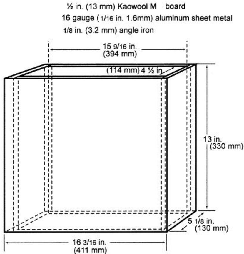
**Figure 2 - Internal Chimney**
