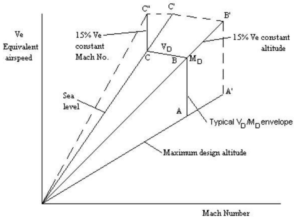
FIGURE 1B MINIMUM FAIL-SAFE CLEARANCE ENVELOPE
