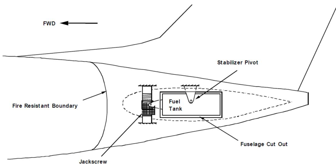
**Figure 3 Example of Distances for Fuel Forward Acting Design Pressure Calculations**
