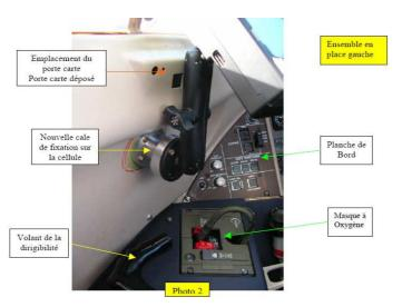
The mounting device consists of a Docking Mount with a latching device which holds the EDU to the mount and provides power and a high speed interface to the unit by means of the EDU-EEMU/EEMU interface cable.
