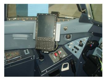
The following shows the installation with the keyboard stowed:
