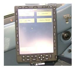
The EDU has a fully dimmable display, a "film-on-glass" touch-sensitive screen, and backlit line select keys (LSKs) providing quick access to specific functions.
