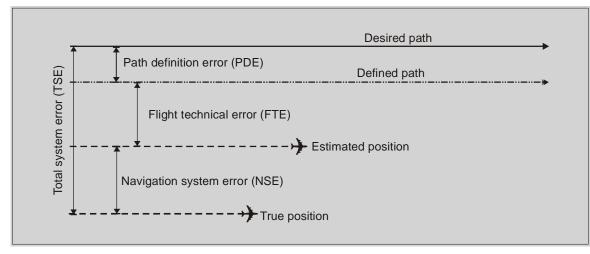
The cross-track and along-track lateral TSE of the aircraft area navigation system should be within  $\pm$  one time the value (in NM) of the required navigation performance (RNP), which depends on the phase of flight (see **Table 2** below), for at least 95 % of the flight time.
