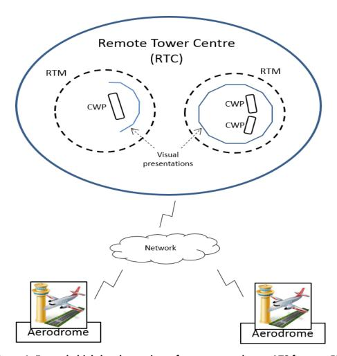
Figure 1: Example high-level overview of remote aerodrome ATS from an RTC
