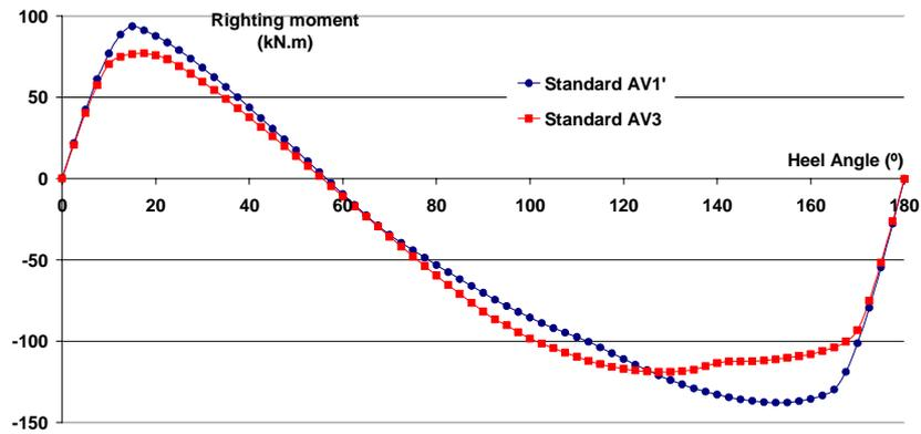
Figure 14: EC225 – Stability curves for the two mass-CG configurations of the analysis
