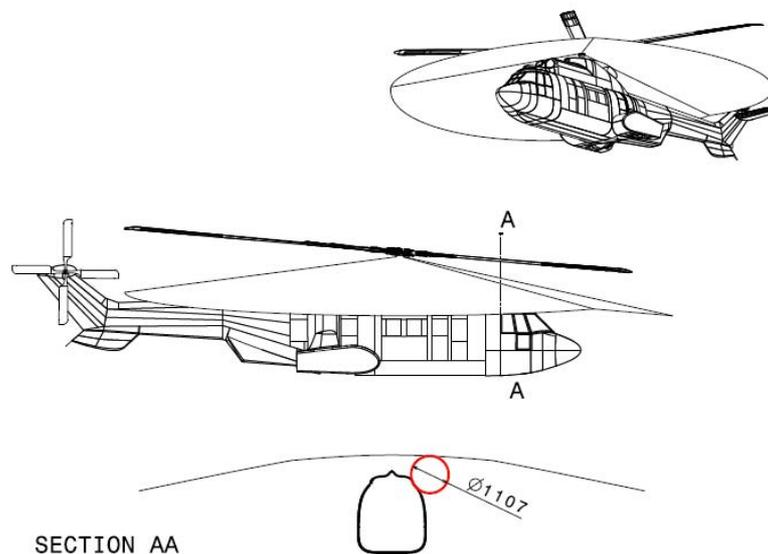
**Figure 24: EC225 – Possible interaction with blades**
