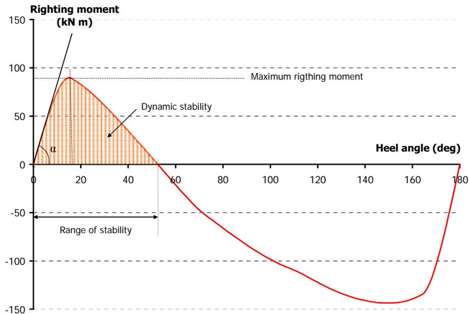
Figure 5: Typical stability curve for a helicopter
