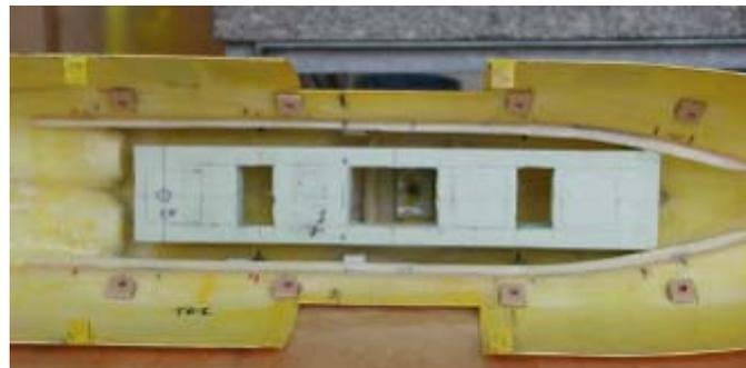
**Foam block representing the inherent buoyancy of the helicopter**
