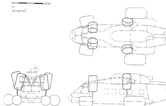
Figure 3: Tethered inflatable floatation units
