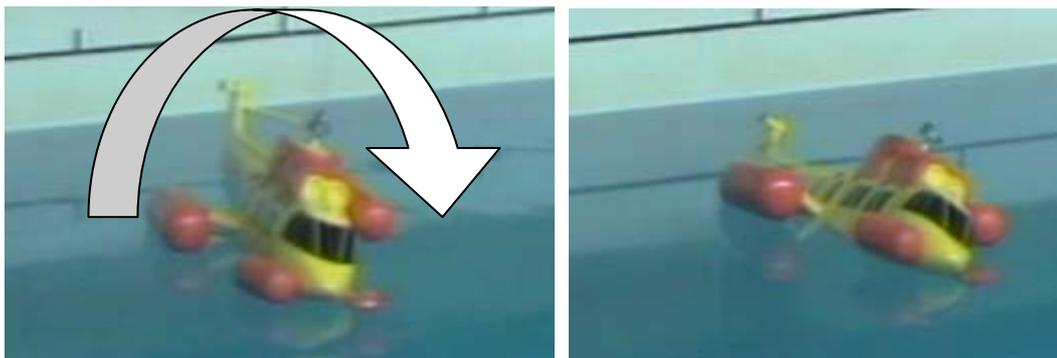
Figure 22: EC225 – Water impact - Config C5 – Rear starboard float removed.
