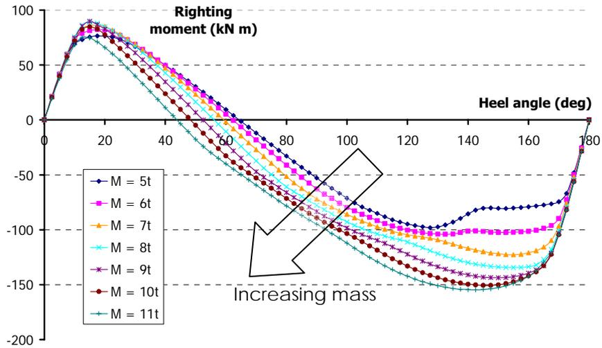
**Figure 11: EC225 - Influence of the mass on the helicopter stability**
