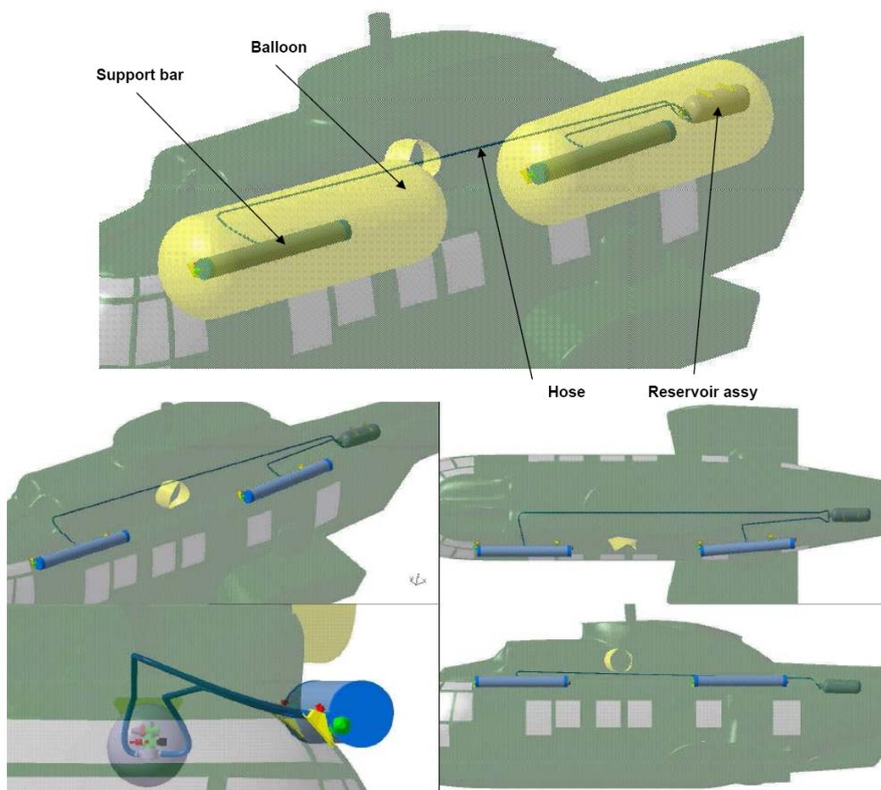
Figure 27: EC225 – Technical solution for the integration of additional EFS
