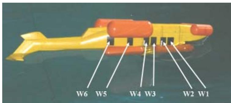
Figure 20: EC225 - Numbering of the windows
