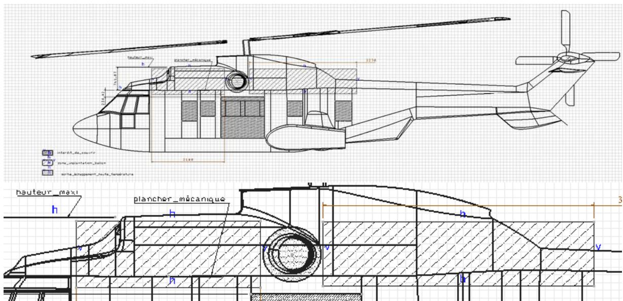
Figure 25: Lateral views of the EC225 with the possible locations of additional floats
