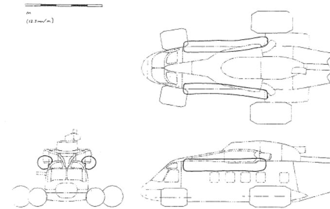
Figure 2: Long buoyancy bags attached along upper cabin wall
