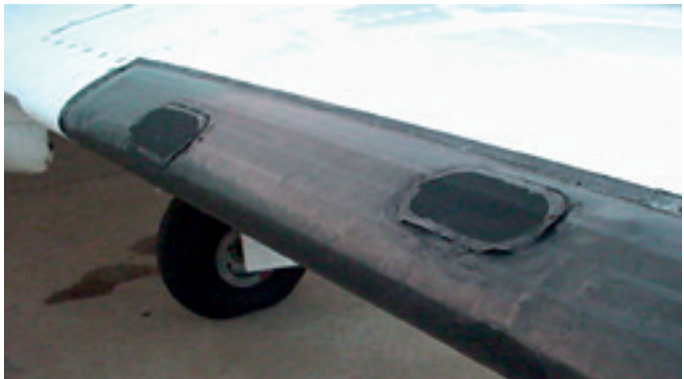
De-Icing Boot with Patch Repairs
