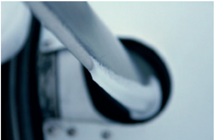
Ice on propeller blade
