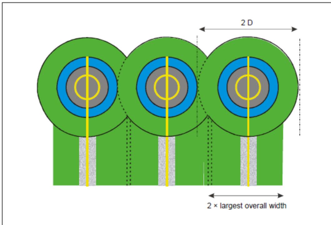
Figure D-3. Helicopter stands designed for hover turns with air taxi-routes/taxiways — non-simultaneous operations
