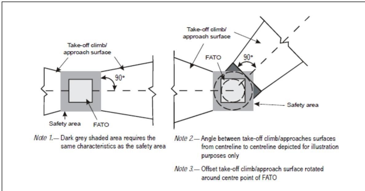
Figure E-1. Obstacle limitation surfaces — Take-off climb and approach surface
