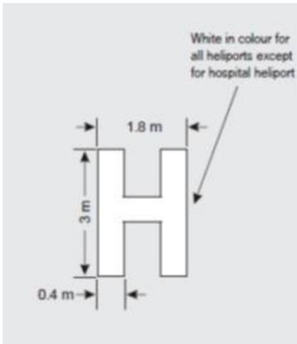
Figure F-3. Heliport identification marking
