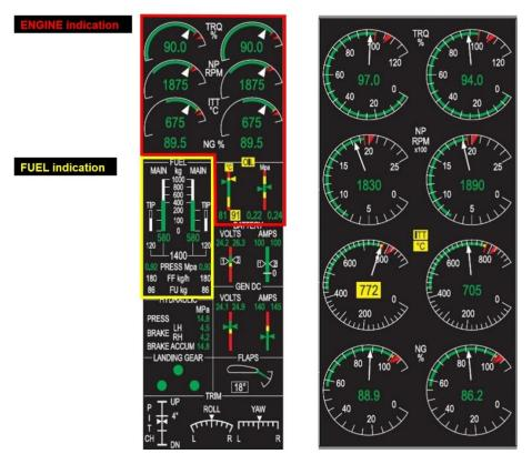
On the primary EIS indicator, where the NG are displayed in only alphanumeric format, the gas generators speed trend can be derived from analog torque indicators and ITT indicators located on EIS just above the NG indications since both torque and ITT are related to gas generator speed. For ground engine starting and in flight starting the use of secondary EIS page with full information about engine parameters is recommended in AFM.
