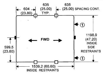
①: During fore and aft testing, an evenly distributed horizontal force equal to 6 times the forward load shall be applied alongside the opposite pallet or container base edge to simulate a possible stack of up to 7 units.
