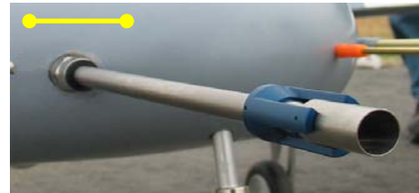
Unbiased aerosol sampling (150 g)
