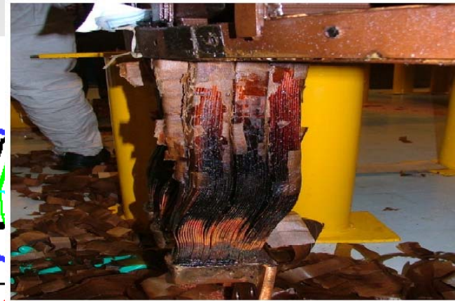
Station 3 Transformer 6 LV exit lead overheating
