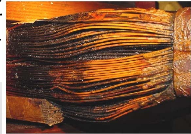
Station 3 Gen. Transformer 5 overheating
