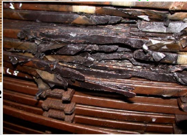
Station 3 Gen Transformer 4 damage
