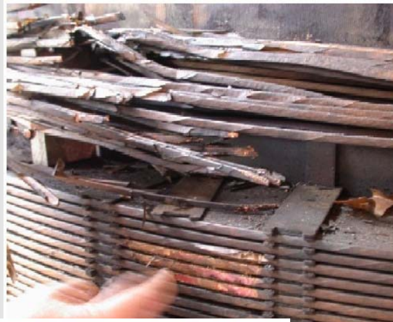
Station 4 Transformer 6 HV winding failure
