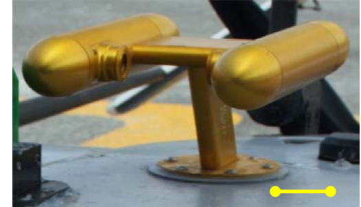
Cloud droplet size & number (1.4 kg)
