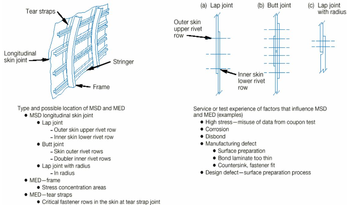
**Figure A2-1 Longitudinal Skin Joints, Frames, and Tear Straps (MSD/MED)**
