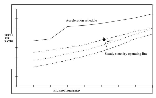
Figure 3 Typical Engine Control Characteristics
