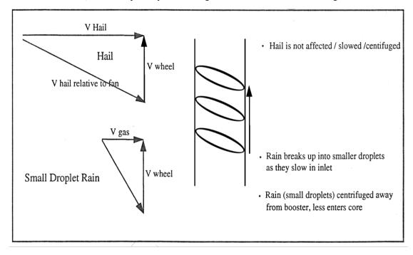
Figure 2 Velocity Vector Diagram
