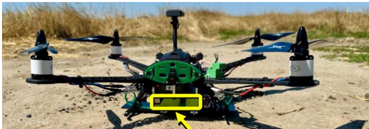
Multicopter test carrier where highlighted module is the onboard monitoring hardware.
