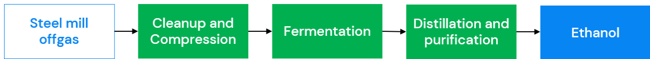
► Figure 5: Exemplar process flow diagram of steel mill offgas to ethanol process
