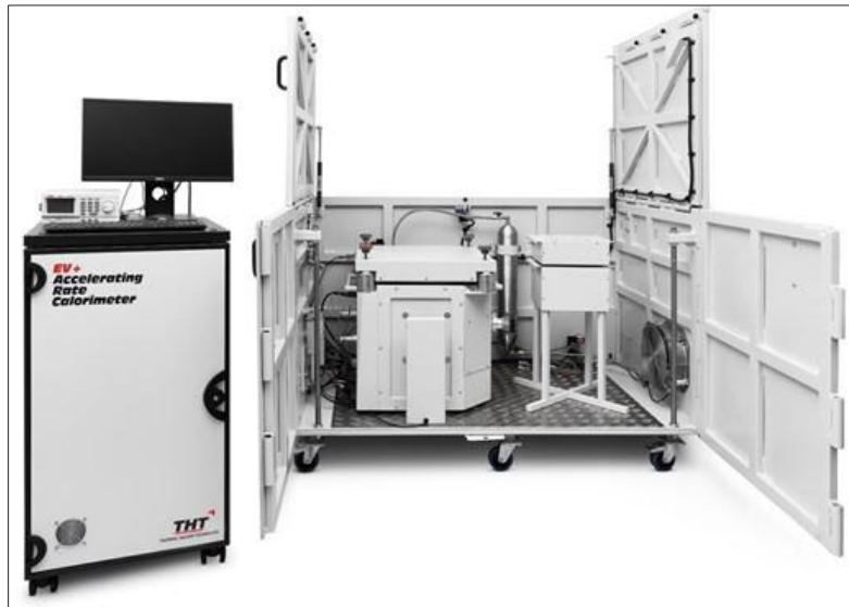
Figure 4: VITO's ARC machine where thermal abuse test can be safely performed and monitored on a cell/battery module
