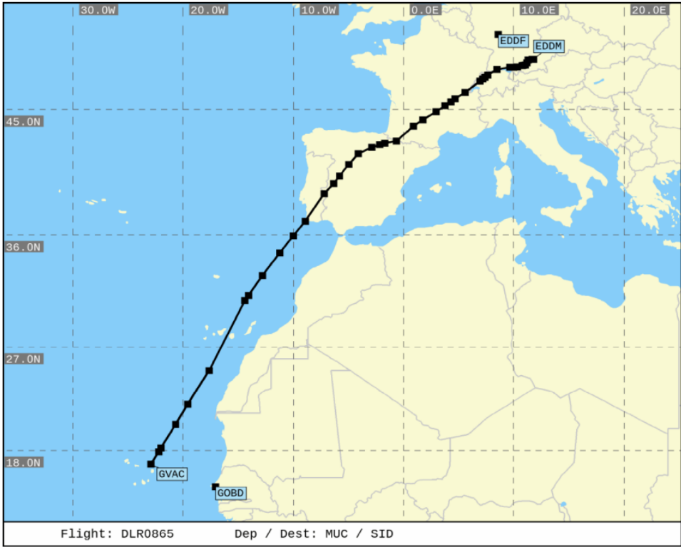
Figure 7: Flight route from Munich to Sal with eMCO entry and exit waypoints and the location where the Engine 2 fire is triggered.
