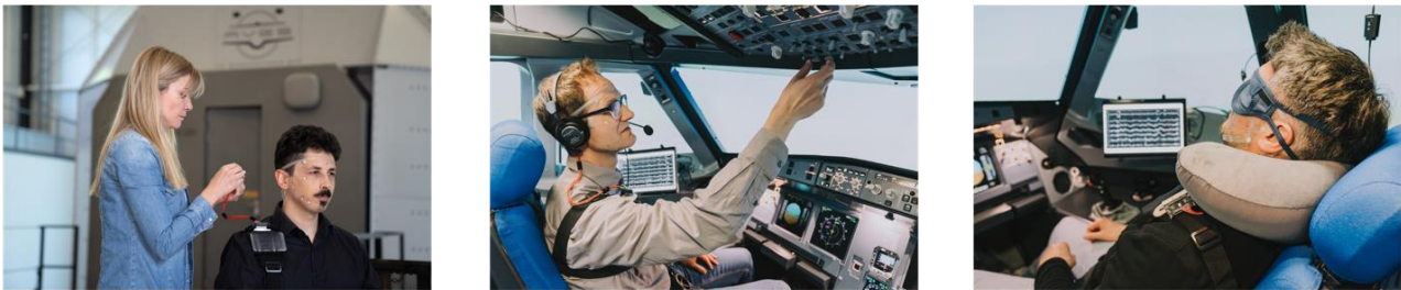
Figure 6: Measuring sleep. Sleep was assessed objectively using an adhesive, soft electrode grid that was attached to the participants' right side of the face. The grid has a comfortable wear, allows for flexible movements and does not interfere with pilots' tasks. ©Fraunhofer IDMT/Anika Bödecker/Leona Hofmann.
