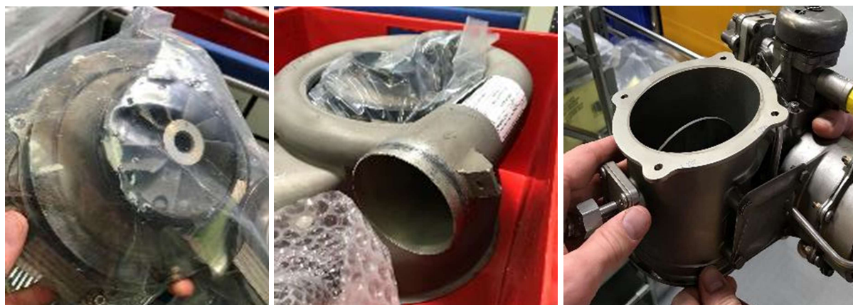
Figure 3 ACM parts (left and middle) and Pressure regulating shut off valve (right) serviced at Honeywell, Bournemouth
