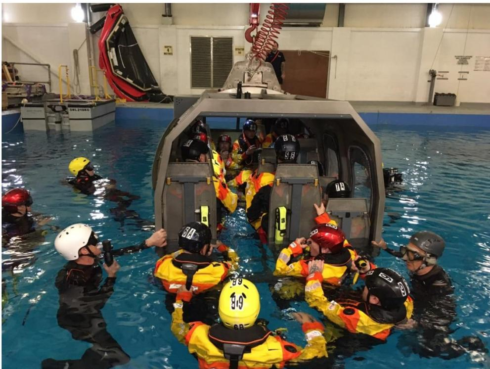
**Figure 3-1 Helicopter simulator loaded with test subjects prior to the 'submersion' trial**
