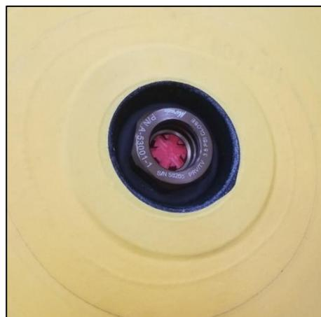
*Figure 6: Representative PRV and PRV Collar*
