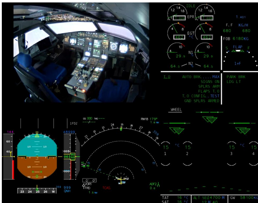
Figure 8: Example configuration of the synchronized video file incl. cockpit rear camera, PFD, ND, and ECAM
