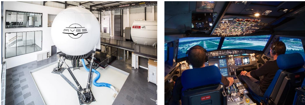
Figure 2: AVES Simulator. Left: The motion platform in the front and one of the fixed platforms in the back. Right: View inside of the Airbus A320 ATRA cockpit.
