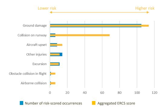
Ground damage was the type of accident most likely to occur in 2018-2022 in case of escalation (real or potential) of the accidents and serious incidents (105 occurrences out of 149). Ground damage also presented the highest cumulated safety risk in the domain (yellow bar).
