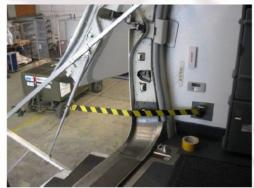
3. In December 2010, **detachable airstairs rails (DAR)** attached to support strut fixed to cabin floor at door L1 & integrated stair rail.
