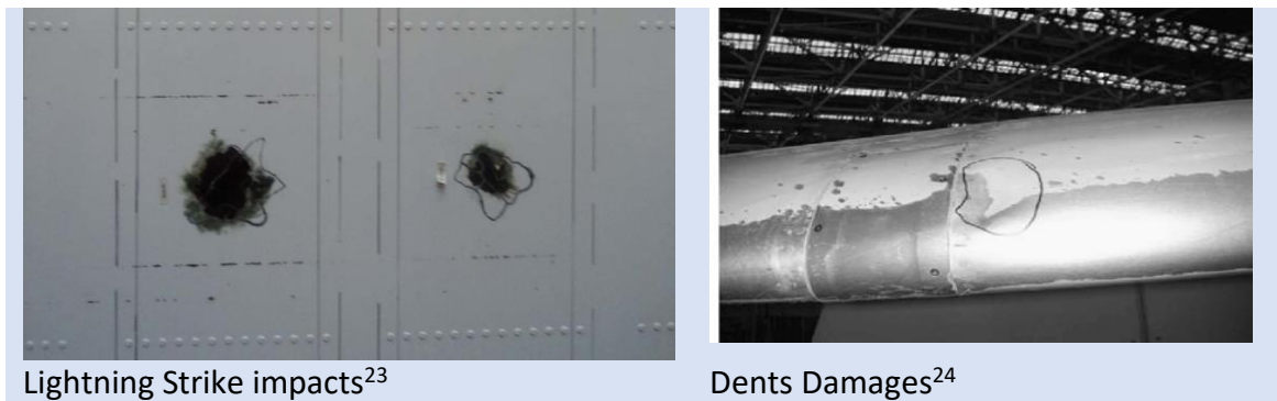
Figure 9. Images showing example damages on an airplane skin.
