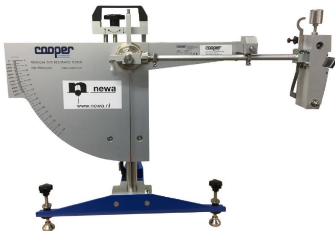
► Figure 4-4 Example of a British Pendulum Tester (Source: NLR)
