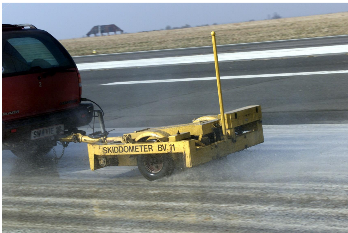
► Figure 4-1 Example of runway friction tester (Source: NASA)
