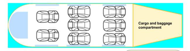
Structural Partition: CS29.561(c) [12g forward] Cargo and Baggage Compartment:
