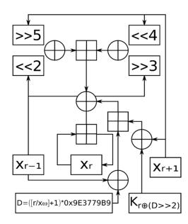
The part of the packet to be scrambled/encrypted with XXTEA shall be a multiple of four bytes as XXTEA works on 32-bit words.
